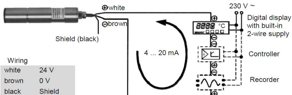
Example for wiring using an external power supply:
