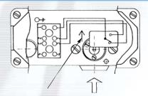
When installing make sure that the flow direction is in accordance with the arrow.
