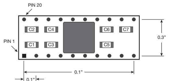
Figure 2 : ADXRS300EB-i Parts Layout
