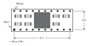
Figure 2 : ADXRS300EB-i Parts Layout
