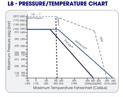
Note: Maximum pressure & temperature is limited to the seat material rating
