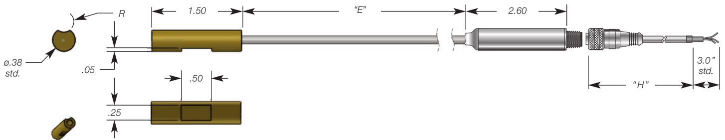
Fig3. Mechanical Dimensions of an R344 with a radius option.
