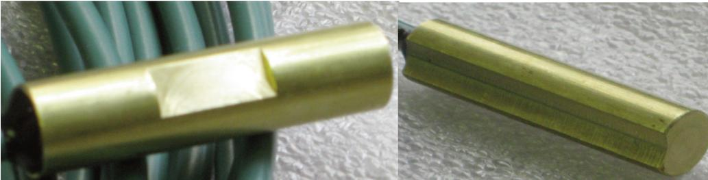
Fig 2. A enlarged view of the brass RTD housing
