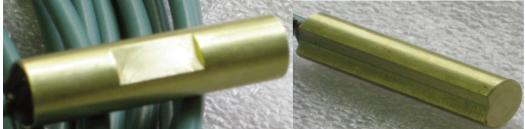
Fig 2. A enlarged view of the brass RTD housing
