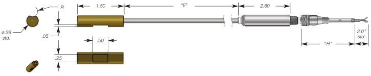
Fig3. Mechanical Dimensions of an R344 with a radius option.
