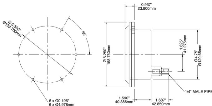
GE® is a registered trademark of General Electric. Gauges manufactured to GE® Drawing U175X.
