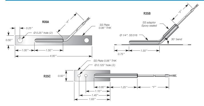
INTEMPCO R35 series surface temperature resistance element is designed to be cemented, clamped or bolted to a surface for temperature measurement. A specially designed moisture seal permits operation in extremely adverse conditions such as may be encountered on cooling equipment and cold water pipes. Teflon insulation and high temperature epoxy permit use at temperatures as high as 200 °C (392 °F).
