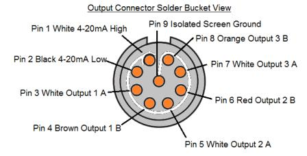
Figure 15 Output Wiring
