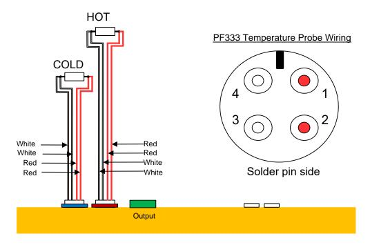
Figure 14 PF333 Temperature Probe Wiring
