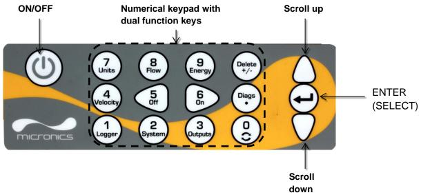
Figure 6 Portaflow keypad
