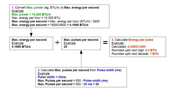
How to calculate a suitable Energy per pulse value from Maximum power and Pulse width (Metric)
