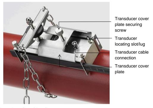
Figure 11 Transducer in guide rail
