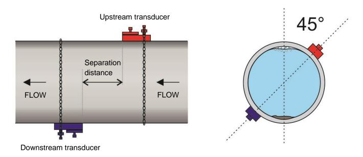
Figure 12 Transducer locations for Diagonal Mode
