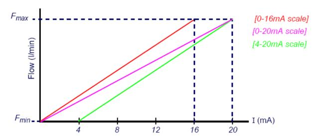
To calculate the flow rate (I/min) for a measured current (mA) then:
