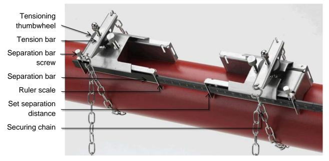
Figure 9 Guide rail assembly (Reflex Mode)
