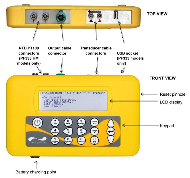
Figure 5 Portaflow unit (PF333HM model shown)
