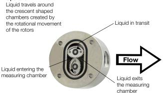
The positive displacement flow technology allows for precise flow measurement of most clean liquids regardless of the media's conductivity. Other liquid properties also have a minimal effect on the performance of this type of meter. Flow profile conditioning is not required, as with alternative flow technology options, making oval gear installations simple to install in tight spaces and at a economical price.
