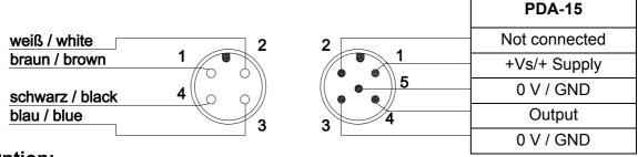
Option: Plug with cable ZUB-KAB-12K002 Plug
