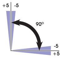
The Quad4 travel stops are designed to absorb the maximum rated torque of the actuator and the maximum impact loads associated with the recommended stroke speed.
