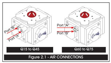
Pressure entering port A into the center chamber pushes the pistons outward and rotates the pinion counter clockwise (CCW), normally the opening direction for valves.
