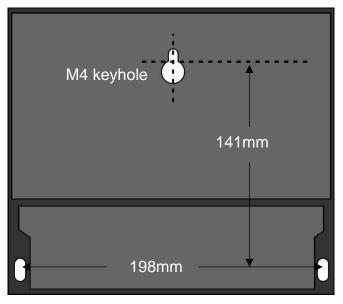
Figure 7 UF3300 mounting dimensions
