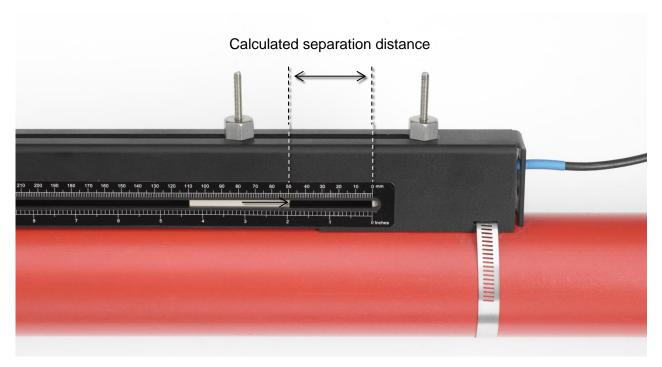
Figure 16 Settinging transducer separation
