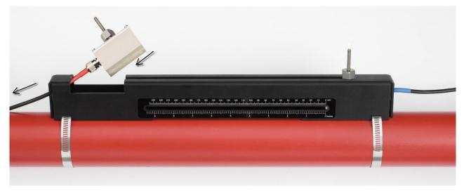
Figure 15 Installing upstream transducer (red)
