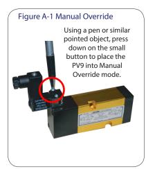
MANUAL OVERRIDE : Use of the manual override will by-pass automatic operation. This function is helpful in the event that the valve must be cycled when electrical supply is unavailable. Press down on the button with a pen or similar pointed object to place the unit in Manual Override. Refer to Figure A-1 above.
