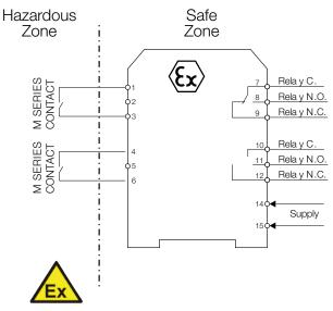
KFD2-SR2-Ex2.W supply:  $20...30 V_{DC}$ KFA6-SR2-Ex2.W supply: 207...253 V<sub>AC</sub>
