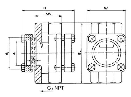
Dimensions (material grey cast iron) for pressure rating PN 16
