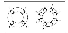
**Torques of cover flange screws [in Nm ]** for lubricated screws and for standard seals made of graphite with stainless steel reinforcement:
