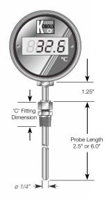
Note: For exact immersion depth, subtract length of fitting "C" from probe length
