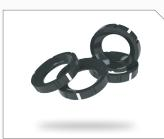
A carbon-infused TFM is the seat of choice for valves used in steam or thermal fluid applications. SupraLon™ has a temperature range of up to 650°F at 30 psig.
