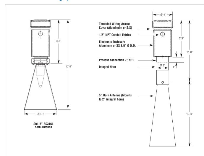
3 and 4 wire Radar Level Sensor
